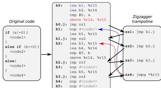
Figure 4: Zigzagger branch obfuscation example (from [42]).
