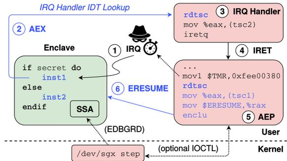
Figure 5: Enhanced SGX-Step framework for precise IRQ latency measurements (blue path) on Intel x86 platforms.
