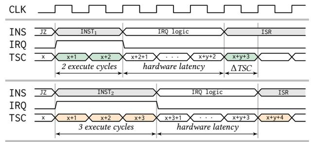
**Figure 2: Interrupt latency leaks information about the instruction that was executing at the time of IRQ arrival.**
