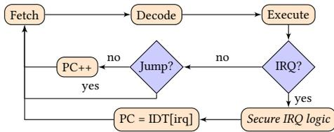
**Figure 1: A processor fetches, decodes, and executes the instruction referred by the Program Counter (PC) register.**
